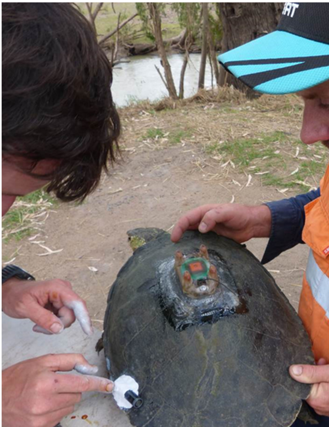
Figure 4 Attachment of SPLASH10 GPS satellite tag and Vemco V13tp acoustic transmitter on an adult female white-throated snapping turtle
