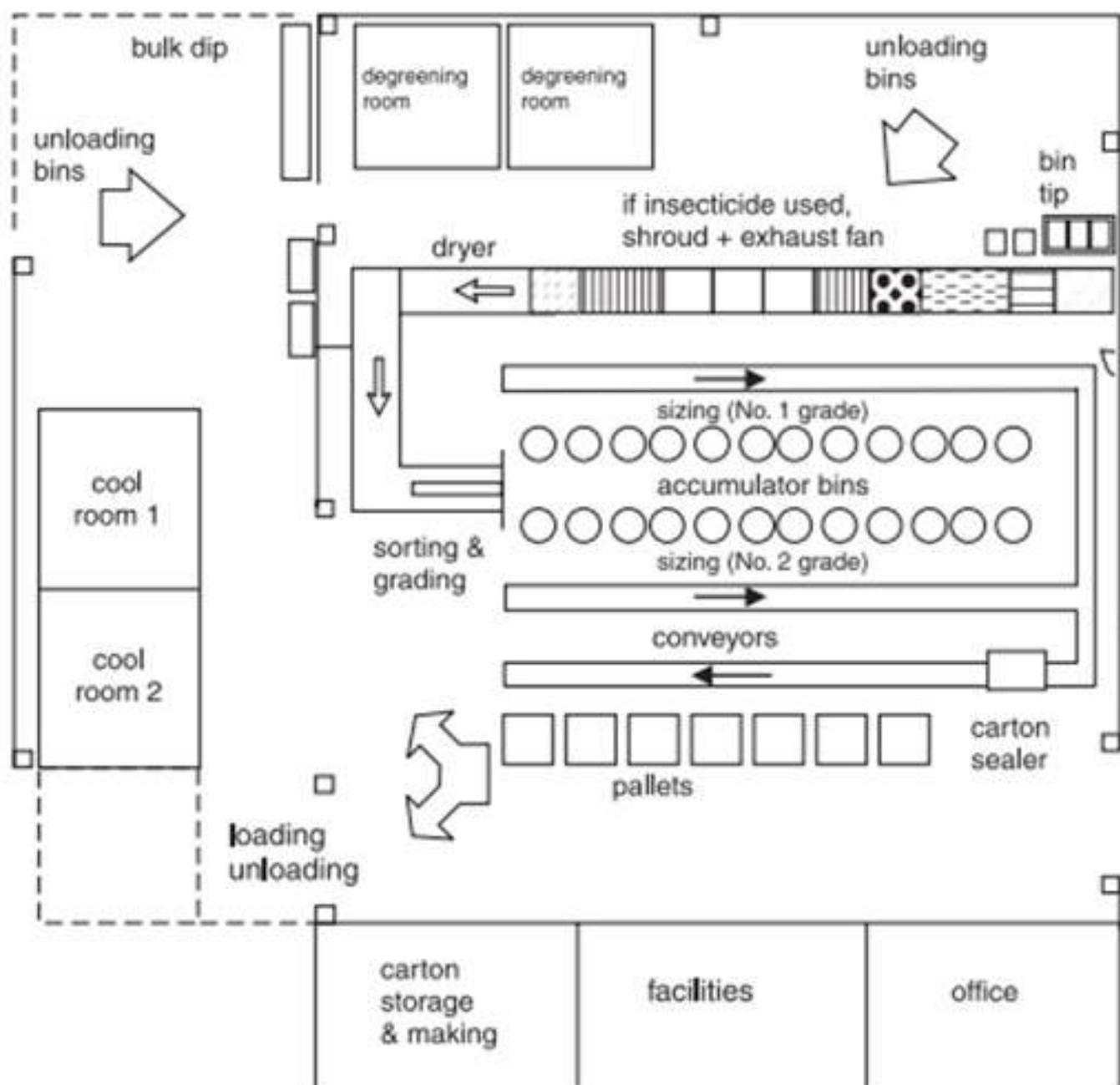
LEGEND: Crop Feed Pre-sort Dip tank Wash off Spinoff Rollers Spare Fungicide (+insecticide where necessary) Wax
