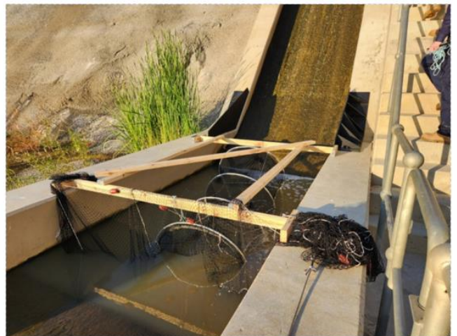
Plate 2.1 Turtle passage capture techniques: cathedral traps at upstream approach channel (top left); seine netting in stilling basin (top right); muddling in resting pools (bottom left) and modified fyke net in a resting pool (bottom right)
