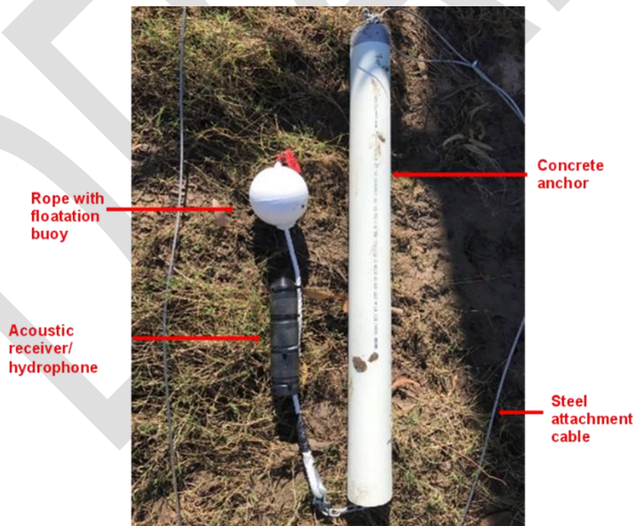
Plate 2.6 Vemco VR2-W underwater acoustic hydrophone mounted to 12 mm rope with floatation buoy and steel attachment cable
