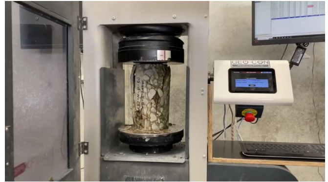
Figure 5: Applying compressive testing to Paradise Dam core samples
