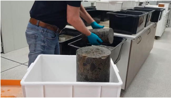
Figure 4: Soaking of Paradise Dam core samples in ethylene glycol
