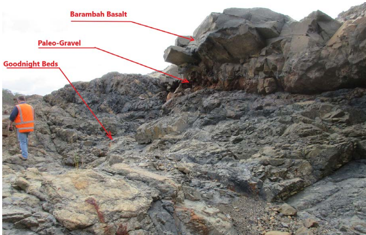
Photo 2.1: Bedrock outcrop on the right side of the river showing three of the primary geological units. A basalt bed is shown at the top of the outcrop. This underlain by the rusty colored, 20 to 30 cm thick paleo-gravel. The Goodnight Beds, with their chaotic fracture patterns, are visible at the base of the outcrop. Despite the variable fracturing of these beds are sound with fair resistance to erosion. Note the curved, sub-horizontal to gently inclined, en-echelon joints in the Goodnight Beds.
