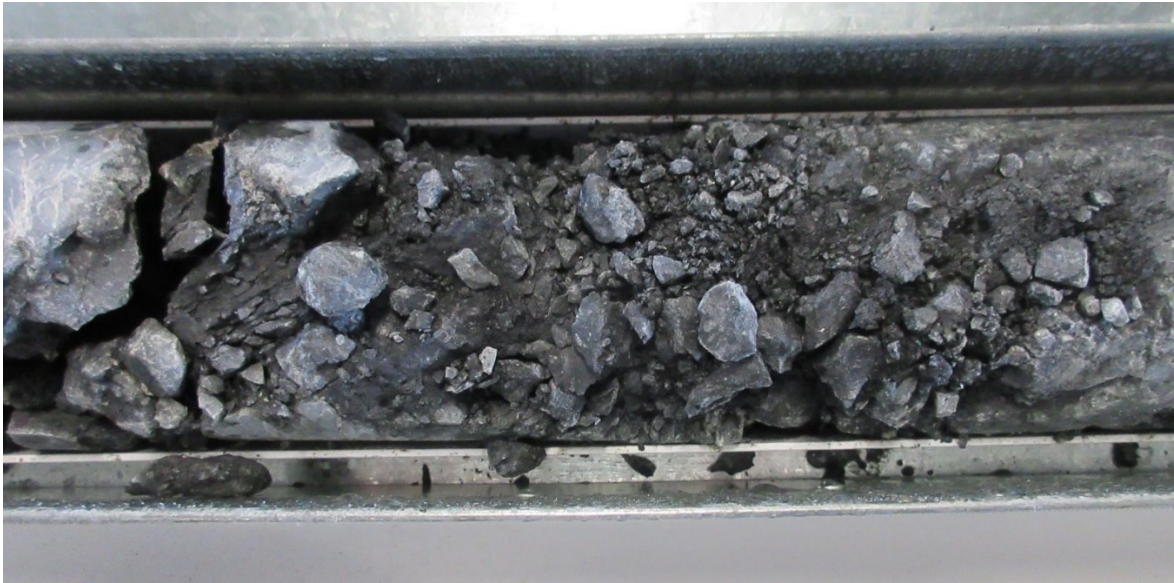
Photo 2.3: Borehole PD-01. Typical sandy gouge with gravel size fragments
