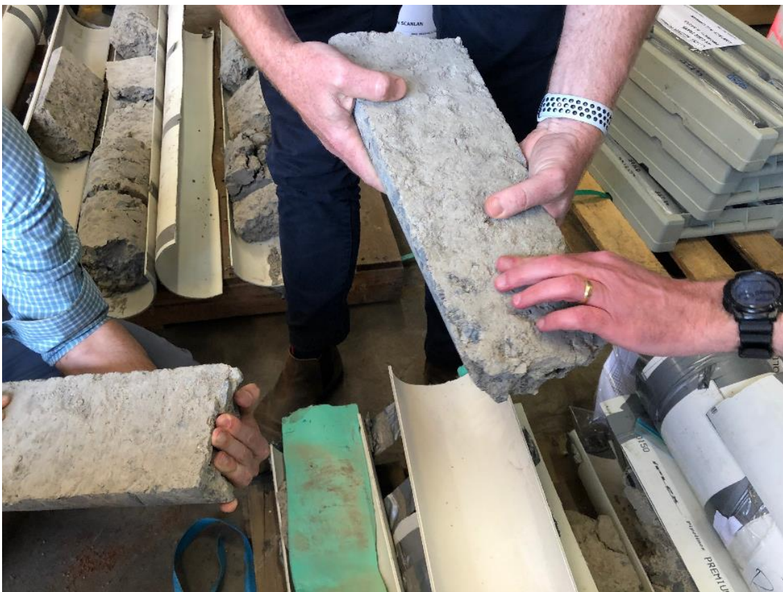
Photo 1 Unbonded RCC Lift Surface
