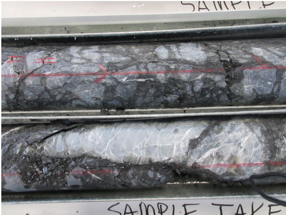
Photo 2.4: Borehole PD-01: Weakly healed breccia. Fracture infilling consist of silica and silt material. is porous and very weak. Sample breaks in breccia fragments when handled
