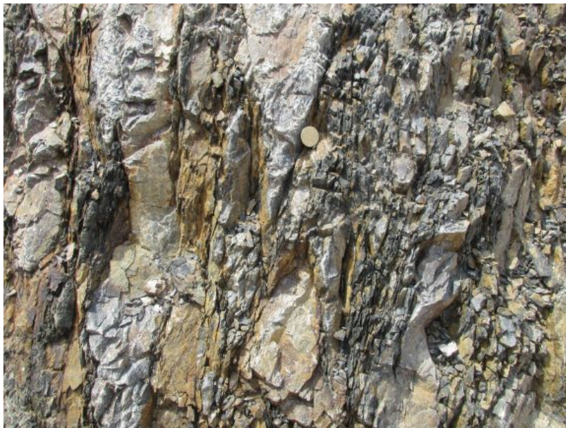
Photo 2.2: Variably sheared meta-arenite and meta-siltstone in the left bank near the Paradise Fault. Shear foliated dark grey carbonaceous meta-siltstone is interlayered with 10 to 20 cm wide nodules and layers of light-colored meta-arenite.
