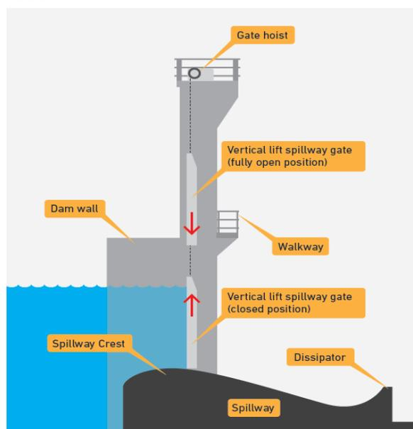
*Image: Cross-section of the E.J. Beardmore Dam spillway looking towards the left bank*
