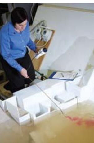
The laboratory is equipped to undertake two and three dimensional hydraulic studies. Two dimensional models are normally constructed in the tilting flume, whilst three dimensional models are contained within bays designed to suit the particular investigation.
