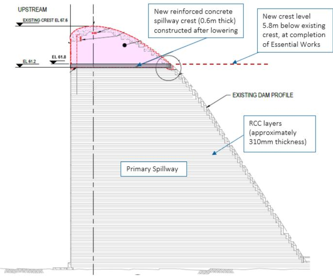
Figure 2 – Section through primary spillway – showing lowered level
