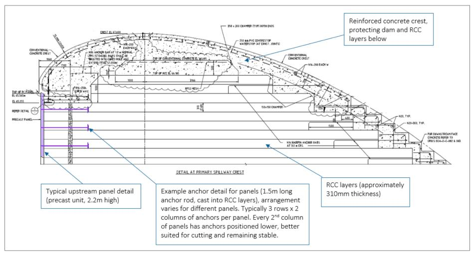
Figure 3 - Primary spillway crest detail, showing precast panels - existing dam
