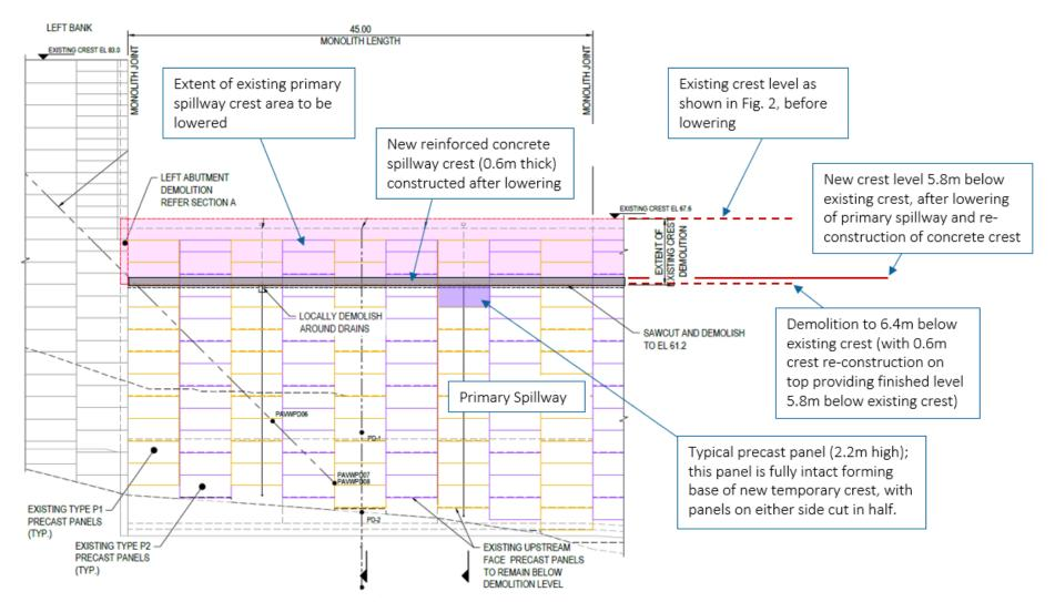
Figure 4 – Upstream face of primary spillway section at left abutment, showing precast panels
